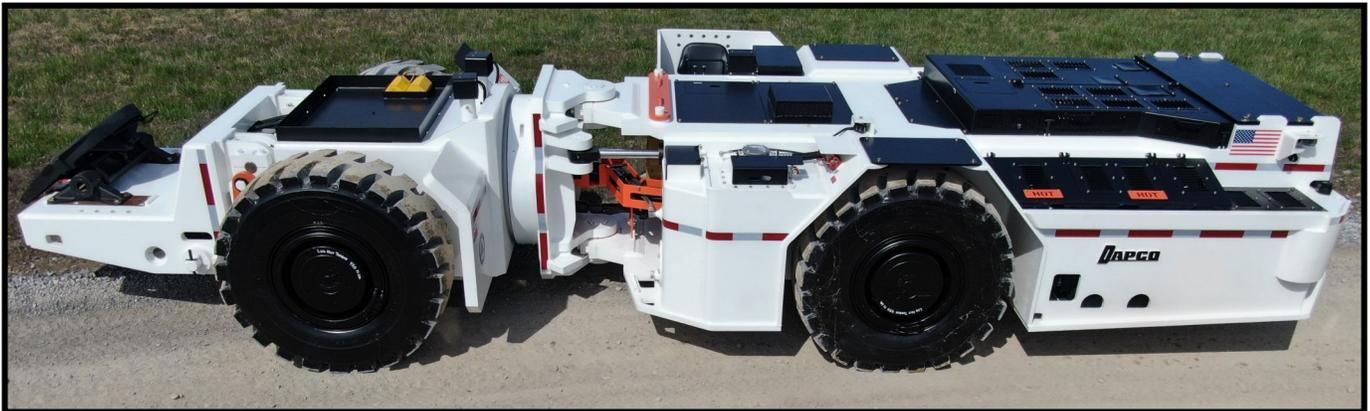
**The DAPCO ST-12100T 100 Ton Tractor is an absolute beast, the big brother to the ST-12 is capable of a 200,000 lb. gross load and the 5th wheel hitch (which has 19" of vertical travel) can support a vertical load of 70,000 lbs. Designed with heavy hauling in mind, this piece of equipment is a must for long wall moves, providing excellent visibility and versatility.**
